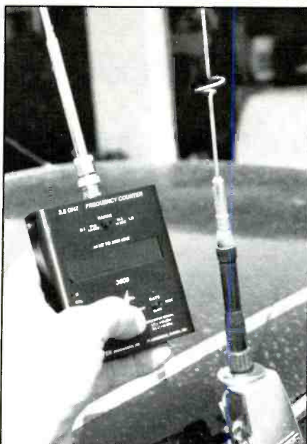
The counter can quickly readout a transmitter's frequency.
