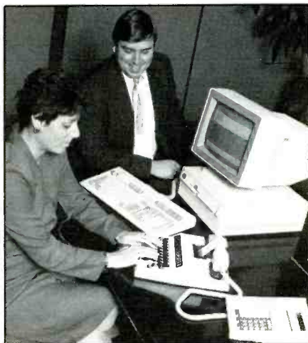
The ROLM telecommunications device for the hearing/speech impaired shown during a demo by two ROLM engineers. The type-writer-like terminal sends/receives written messages.
