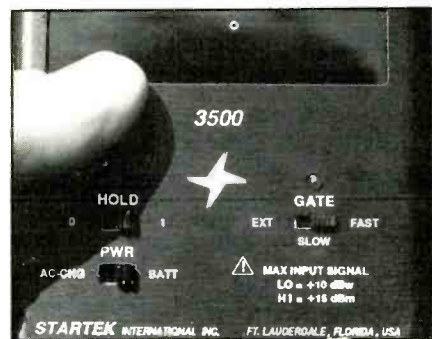
The hold button locks the counted frequency into the display.
