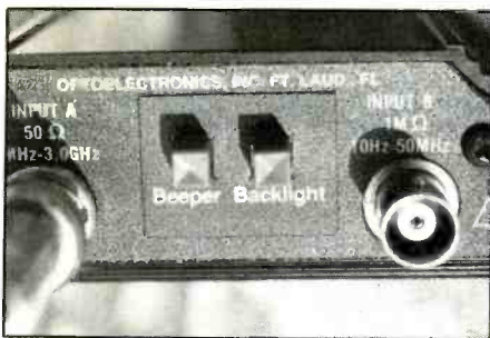
The backlight and beeper option may be re-fitted to most Optoelectronics counters for under $100.
