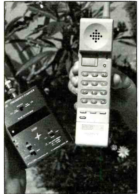
Counting a cordless phone—both antennas must be within a few inches of the reading.
