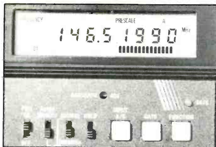
The LCD signal strength bar graph is necessary to track down local signal sources.
